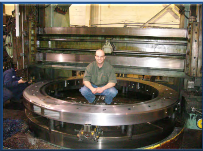
Turbine Bearing Runner Plate, Canada
